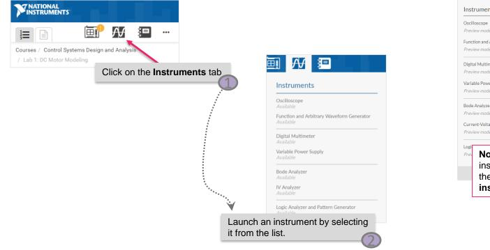
Instruments Preview mode only [?] Function and Arbitrary Waveform Generator Preview mode only [?] Digital Multimeter Variable Power Supply Bode Analyzer Current-Voltage Analyzer Preview mode only [?] Note: You must connect to the instrument on the **Device** tab before they will be available on the instruments tab.
